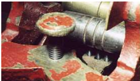
All later embossing registers used Vail's design of a steel pen with a grooved roller.
