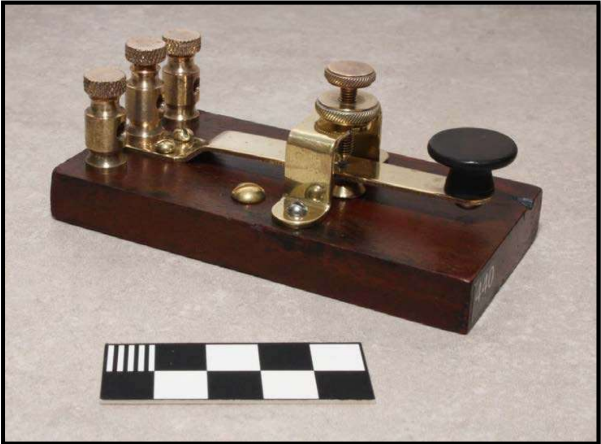
Figure 5 Strap key for telegraphy use. Most likely by J.H. Bunnell. Size 10cm x 5cm.
