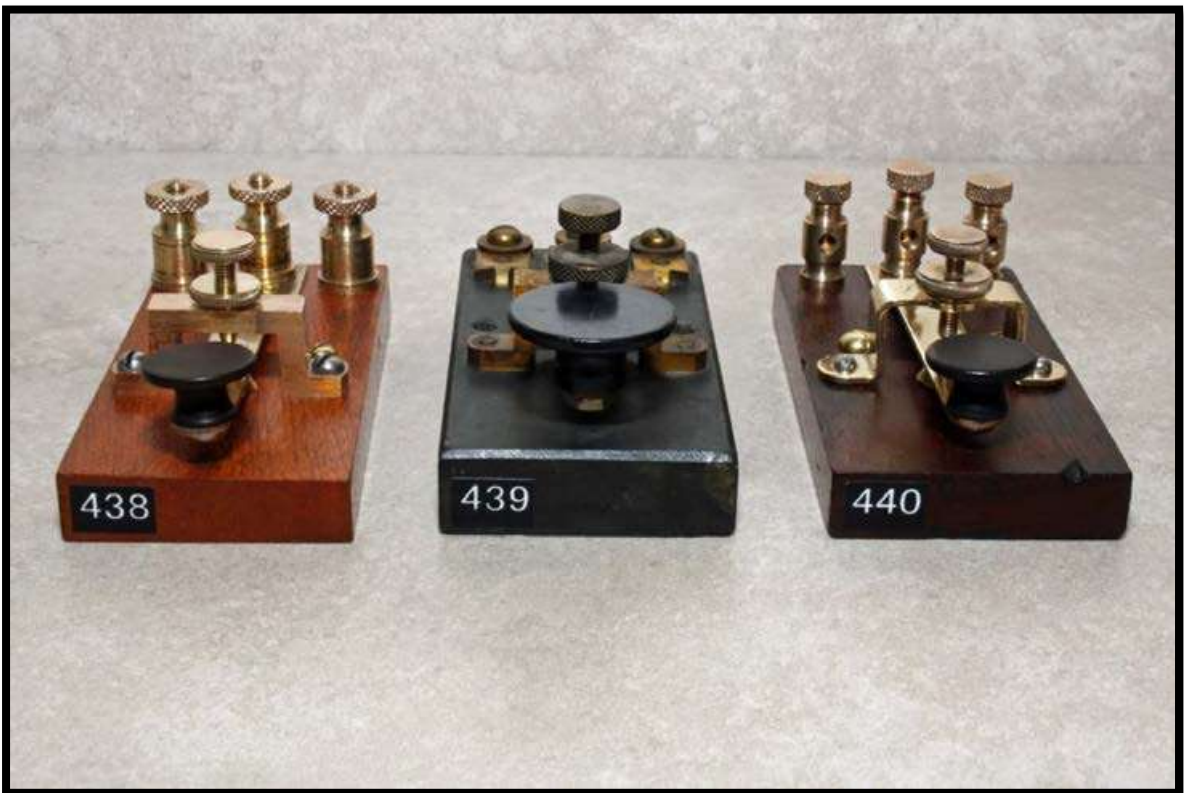
Figure 6 Telegraphy strap keys. J.H. Bunnell key on stone base at centre. Size 10cm x 5cm.
