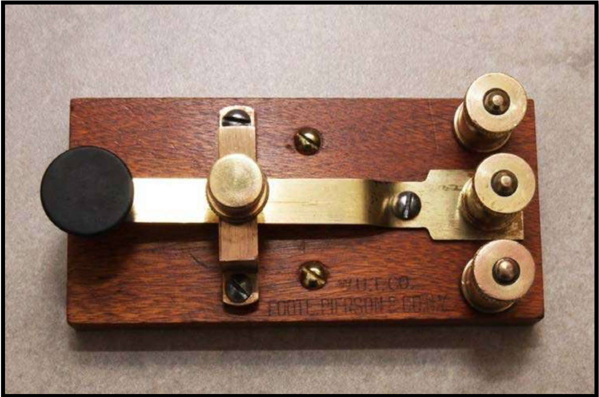
Figure 7 Foote.Pierson & Co. N.Y. strap key for Western Union Telegraph Company use.
