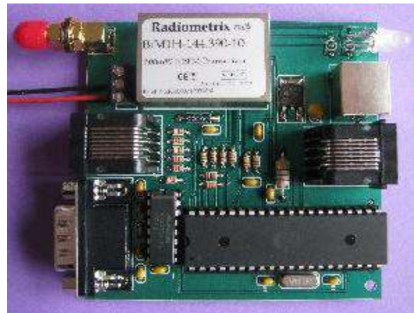
Byonics MicroTrak 4 configured as a digipeater
