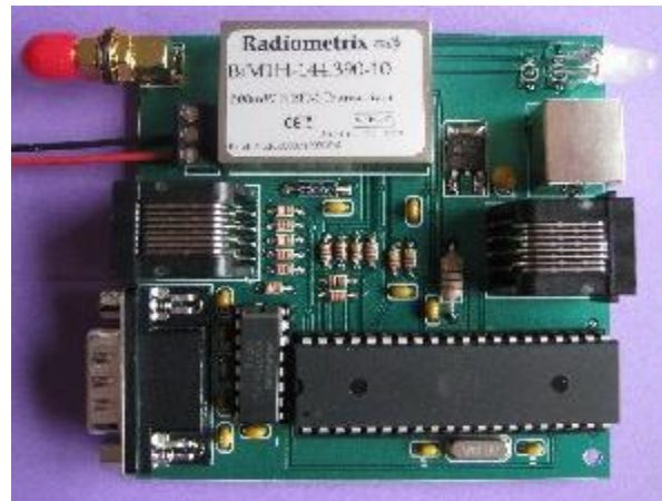
Byonics MicroTrak 4 configured as a digipeater
