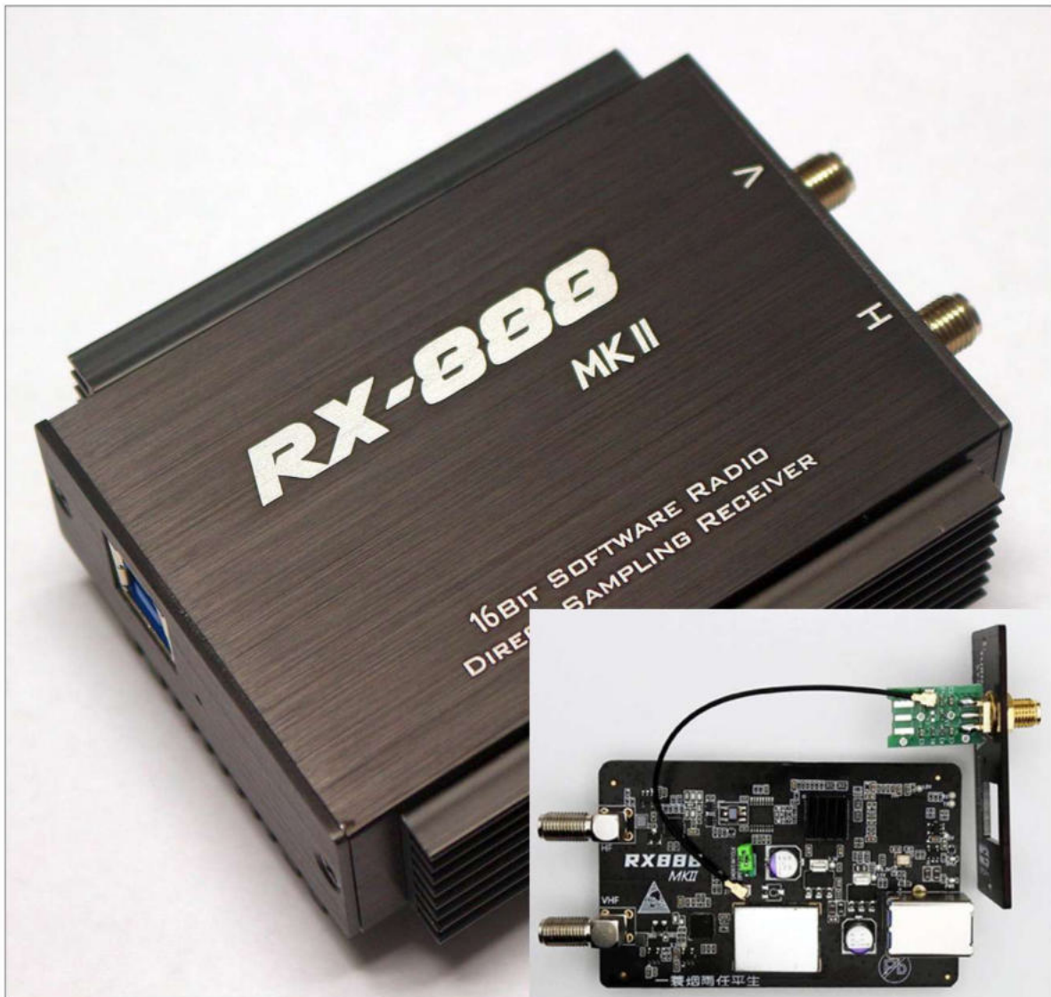
Figure 1 — RX-888 MKII SDR with Turn Island Systems GPS clock kit. Credit: rx-888.com and Turn Island Systems.
