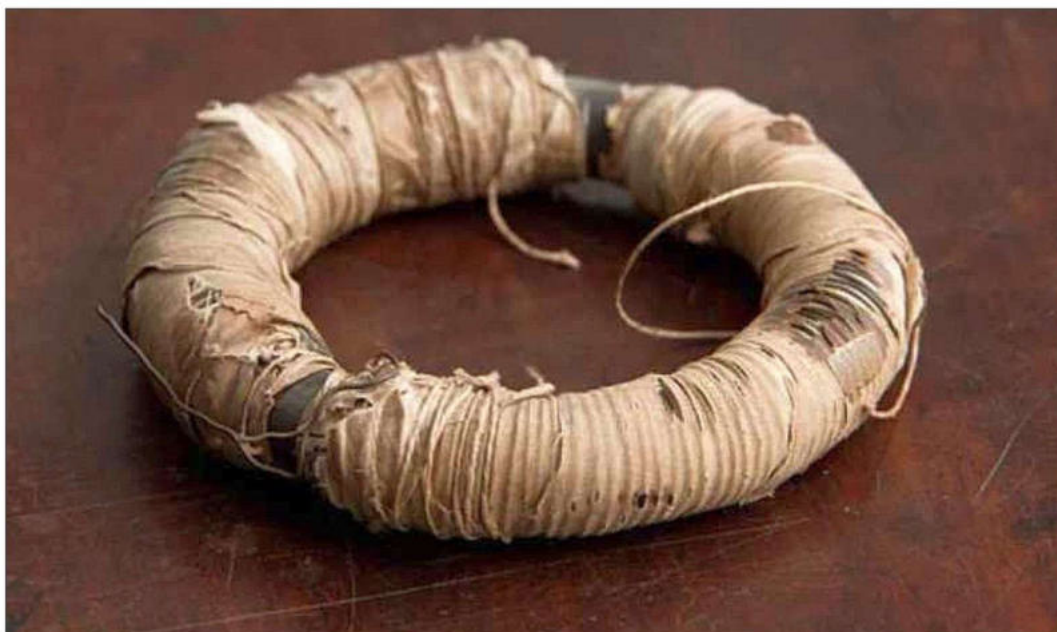
Figure 2A: Faraday's Induction Ring — The nearly two-hundred-year-old Faraday proto-transformer was painstakingly hand-wound. Credit: Royal Institution of London.
