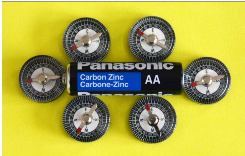
Figure 2B: Magnetic Field around an AA Carbon-Zinc Cell
