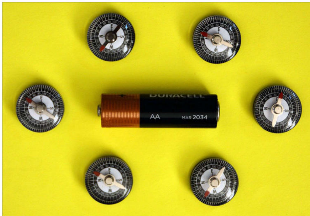
Figure 2C: Magnetic Field around an Alkaline AA Cell
