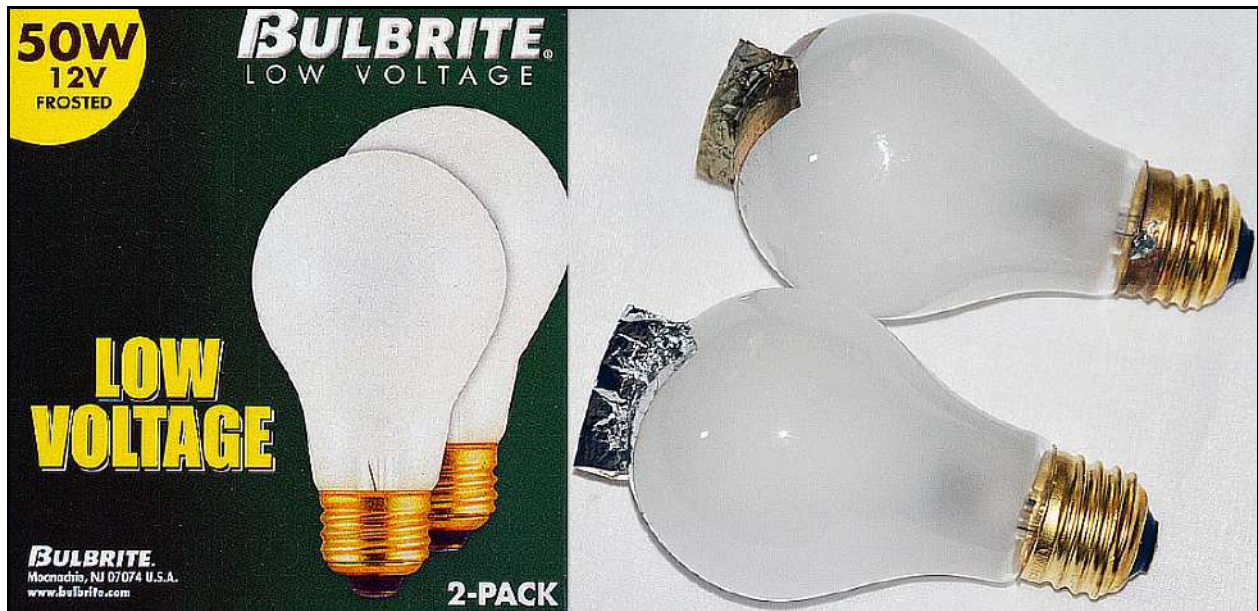
Low voltage light bulbs with aluminum and copper foil external “plates”
